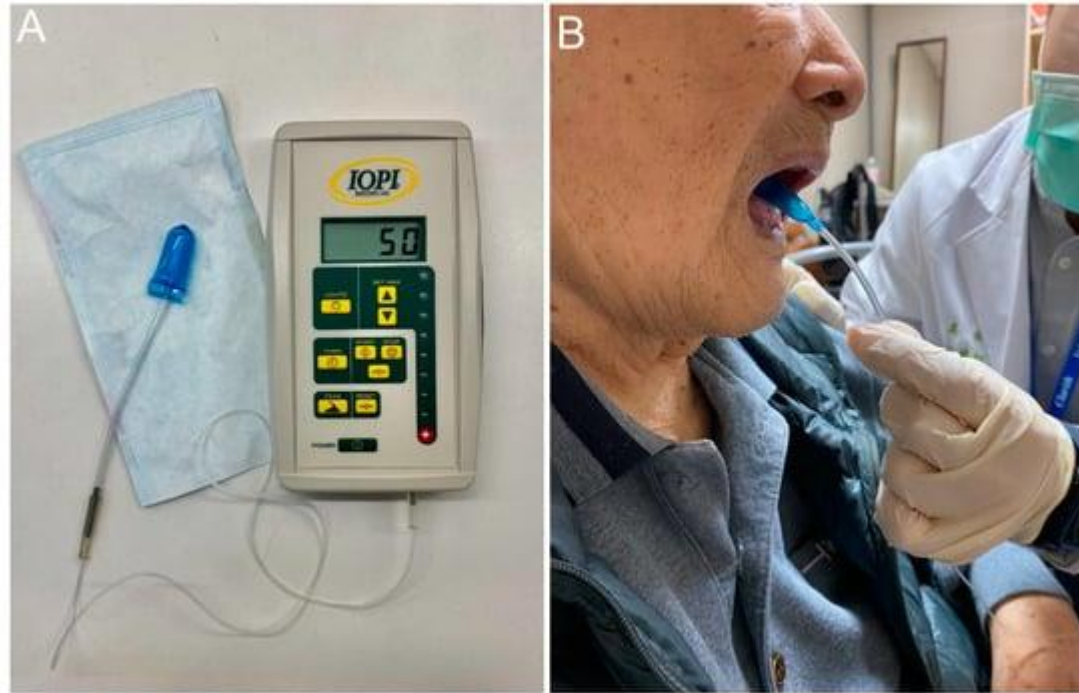
The Iowa oral performance instrument ( A ) and how it is used for obtaining maximal tongue pressure ( B ).
